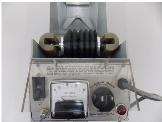
Figura 10. ISCP dielectric strength tested up to 35 kV.
